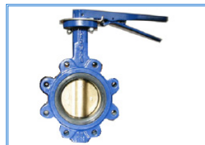
BL-1000-22DBL (DEL) 200 WOG, Buna(DB) or EPDM (DE) Seat, SS Disc
