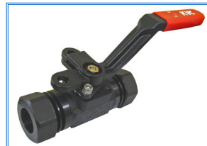
C-336SS(ST)-LF2 , Class 2500, 6000 WOG, 3-Piece, Forged Steel, Mounting Pad, Extended Socket Weld Ends(C-336SS), Extended Socket Weld End x NPT End(C-336ST), 1/4" - 1 1/2" - Full Port, 2" - Standard Port
