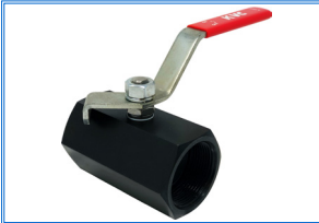
A-122T , 2000 WOG, 1-Piece Reduced Port, NPT Ends, Barstock Body
