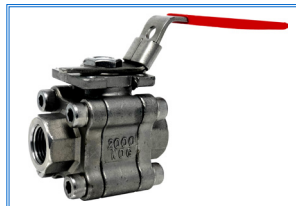
S-362T-F , 2000 WOG, 3-Piece Full Port, NPT Ends , Square Stem, Fire-Safe, ISO 5211 Direct Actuator Mounting Pad
