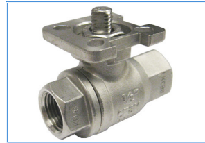
S-231TD , 1000 WOG, 2-Piece Full Port, NPT Ends , Square Stem, ISO 5211 Direct Actuator Mounting Pad
