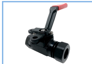
C-333SS(ST)-LF2 , Class 1500, 3000 WOG, 3-Piece, Forged Steel, Mounting Pad, Extended Socket Weld Ends(C-333SS), Extended Socket Weld End x NPT End(C-333ST), 1/4" - 1 1/2" - Full Port, 2" - Standard Port
