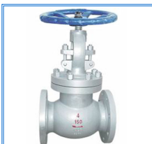
276-CS-150 , Globe Valve, Class 150, F-F Flanged Ends, Bolted Bonnet, 13Cr/HF Iron, WCB Body & Bonnet
