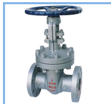
272-CS-300 , Gate Valve, Class 300, F-F Flanged Ends, Bolted Bonnet, 13Cr/HF Iron
