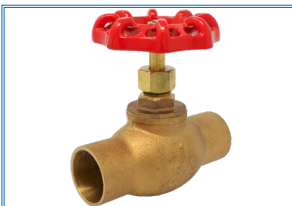
112 , Globe Valve, Class 150, PTFE Disc, Union Bonnet, Solder Joint Ends
