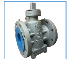
282-CS-150 , Balancing Plug Valve, Class 150, F-F Flanged Ends, Bolted Bonnet, 13Cr/HF Trim WCB Body & Bonnet
