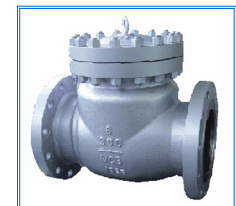
278-CS-300 , Swing Check Valve, Class 300, F-F Flanged Ends, Bolted Bonnet, 13Cr/HF Iron, WCB Body & Bonnet
