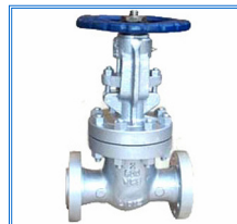
272-CS-600 , Gate Valve, Class 600, F-F Flanged Ends, Bolted Bonnet, 13Cr/HF Iron
